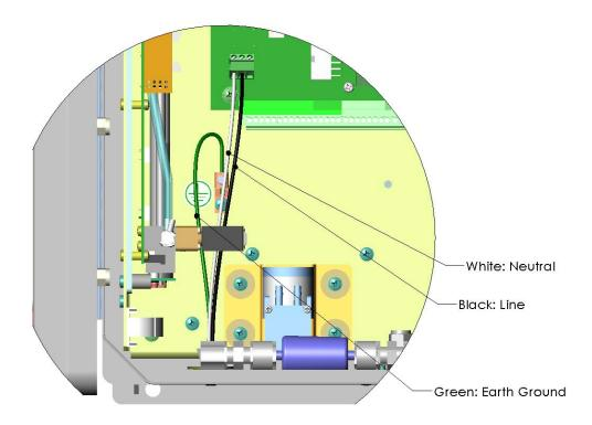
Figure 4-1: NEMA AC Power Connection to Monitor
